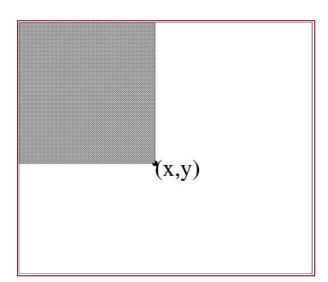
Definition: The integral image at location (x,y) contains the sum of the pixels above and to the left of (x,y), inclusive:
