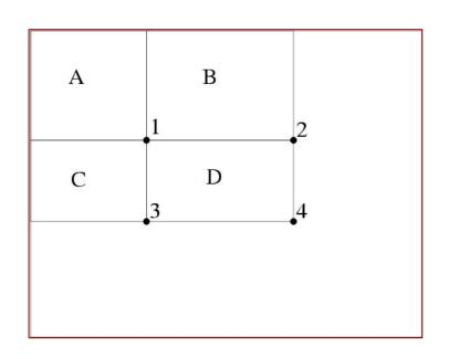
Using the integral image any rectangular sum can be computed in four array references
