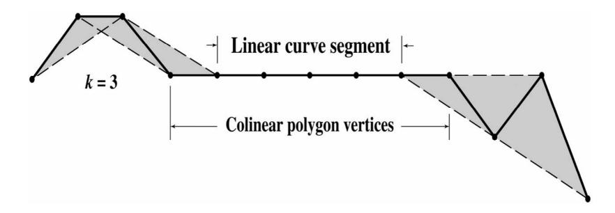
Straight line results start and stop k-2 spans from the ends of the co-linear segments
