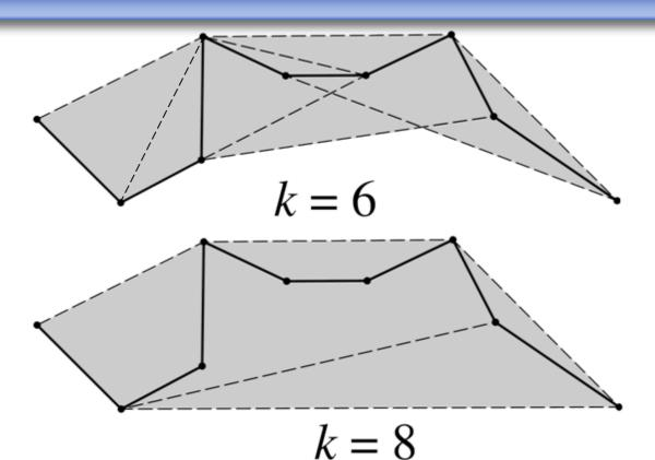
The higher the order the less closely the B-spline curve follows the control polygon
