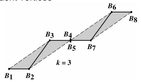
k-1 coincident vertices are required for the curve to pass through the vertices
