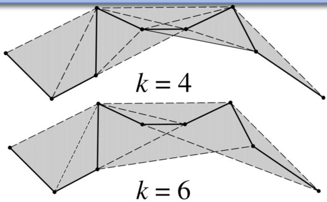
The higher the order the less closely the B-spline curve follows the control polygon
