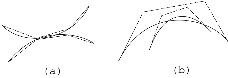
Fig. 5.14. Linear approximation of curves in finding intersections: (a) approximation by linear segments, (b) approximation by polygon
