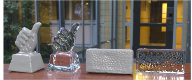
Fig. 10 Reconstruction results and their corresponding rendering results for a trophy object and a brick object with bumpy front surface.
