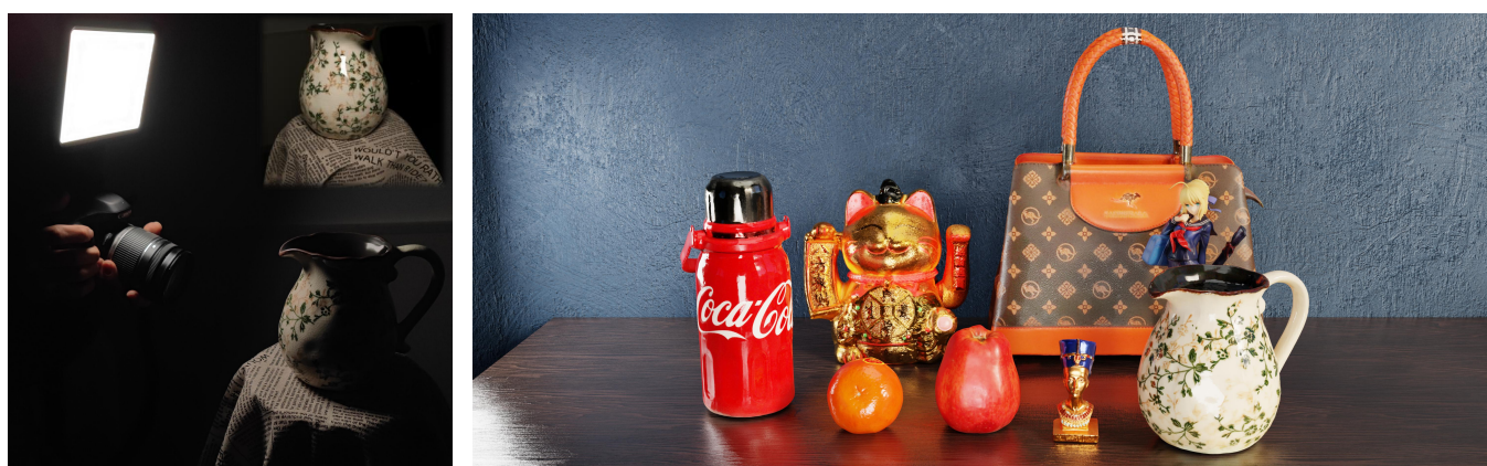
Fig. 1. We investigate active area lighting in inverse rendering to capture the BRDF material and geometry of real-world objects ( left ). Area lighting can be efficient as it samples a broader range of BRDF angles, reducing the number of photos required thanks to better material roughness estimation. For rendering, we compare MC methods to differentiable linearly transformed cosines (LTC). While both can produce high-fidelity relighting ( right ), LTC can be faster.
