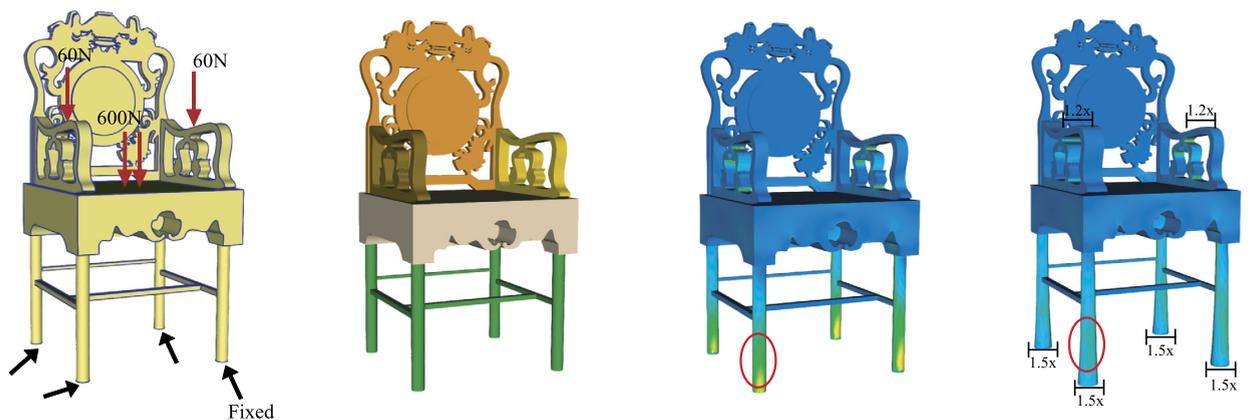
**Fig. 10.** The integration of IWires editing and stress analysis on a chair model. The blue lines on the chair model indicate the extracted wires.
