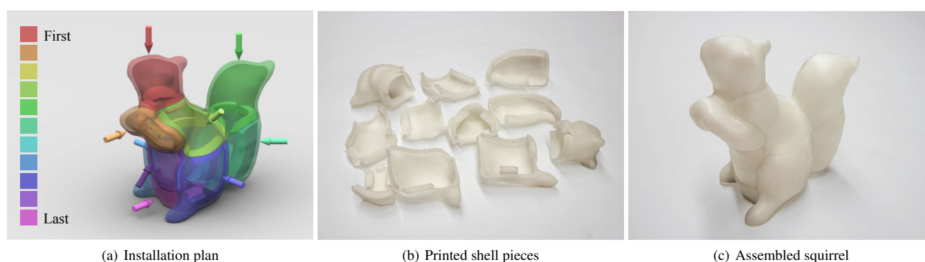
Figure 1: A squirrel example. Our computational system generates interlocking shell pieces from a printable model. Without using glue or screw, the shell pieces in (b), printed by a Form1+ SLA printer, can be securely locked in the assembled configuration as (c) shows. The color pieces and arrows in (a) visualize the installation plan, including both the installation order and the installation directions of the pieces.
