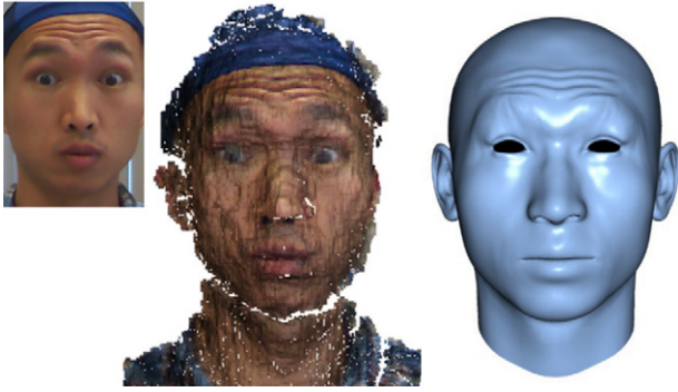
Fig. 1. Top-left: Captured RGB image. Middle: The corresponding Kinect raw depth data using the RGB image as its texture. Right: 3D mesh recovered with wrinkle details using our method.
