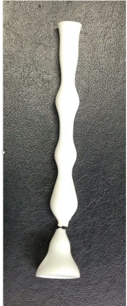
Fig. 14. The 3D printed lamp stand fails and the failure location matches the area where high stress distribution is observed.
