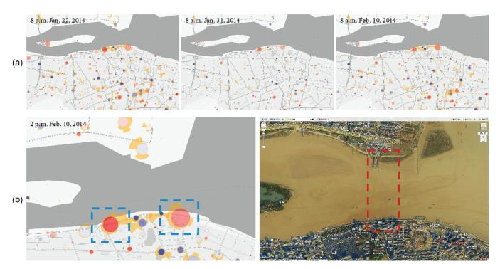
Fig. 2. Visual analysis of human mobility based on cell phone location data [23]. (a) The sunburst views for three different days; (b) The sunburst view for a ferry area and the corresponding image.
