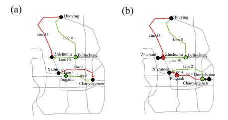
Fig. 3. Examples of minimum travel time paths (red lines) and minimum travel cost paths which take congestion cost into account (green lines) for the Beijing subway network. The black nodes indicate the origins or destinations of passenger trips, and the green and red nodes indicate the transfer stations. (a) Routing adjustments changes a direct path to a path with one transfer. (b) Routing adjustments changes the transfer stations.
