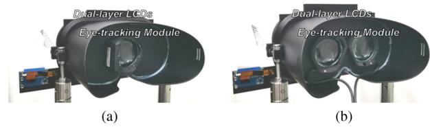
**Fig. 11.** (a) Monocular and (b) binocular prototypes of the foveated display. These prototypes comprise two stacked LCDs and a commercial eye-tracking module, respectively.
