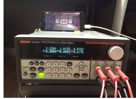
Figure 1: A smartphone with 2.2 GHz 8-core ARM Cortex-A53 CPU and PowerVR G6200 GPU, and a Keithley A2230-30-1 sourcemeter
