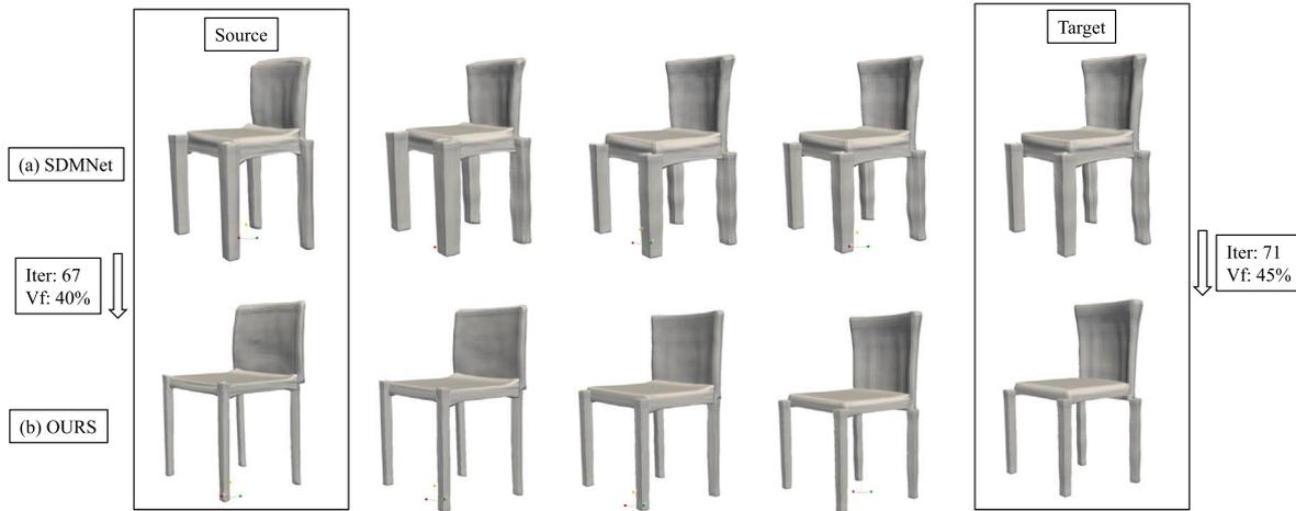
Fig. 6. Comparison of interpolation methods. (a) Top row: SDMNet method interpolation, (b) Bottom row: SATO’s approach, demonstrating lightweight topology optimized shapes. Source and target shapes maintain volume fractions of 40% and 45% respectively.
