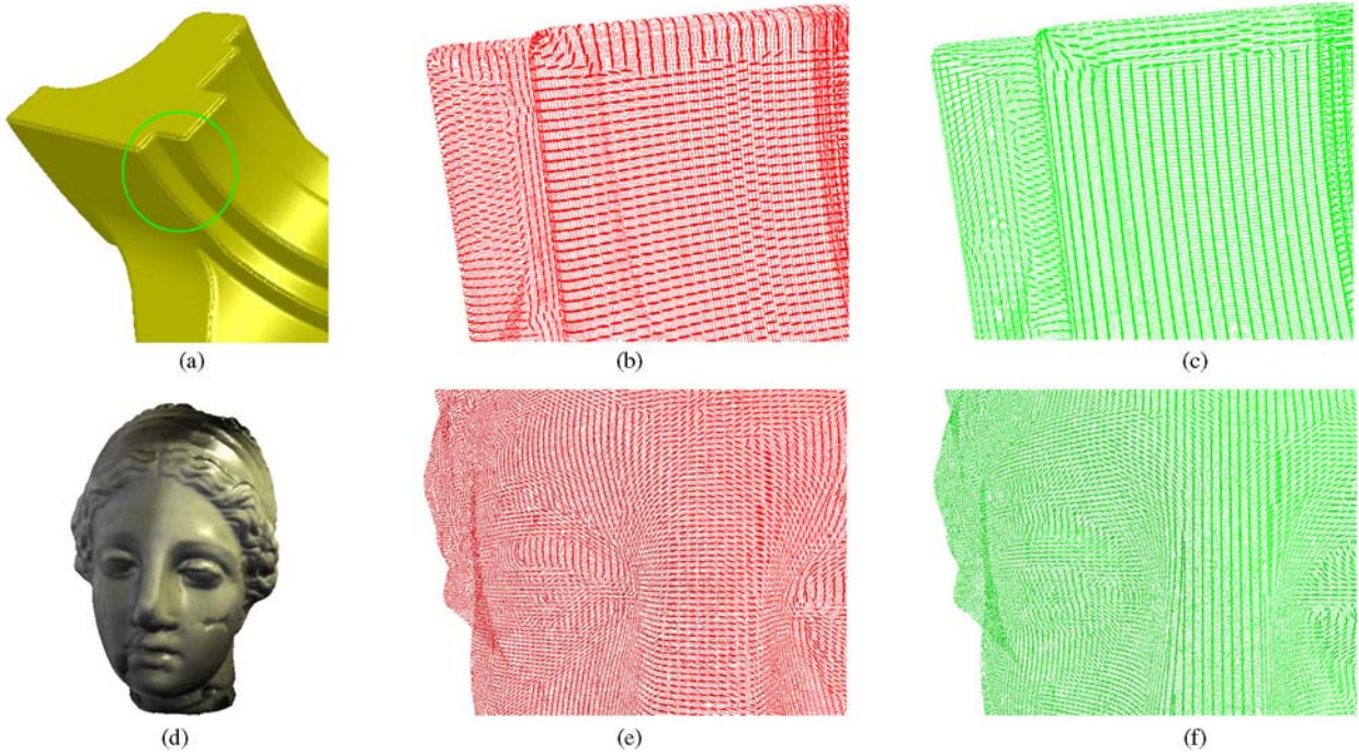
Fig.4. Principal curvature direction estimations by our projection method. (a) Original fandisk model. (b) \kappa_1 -principal directions for a corner of fandisk model. (c) \kappa_2 -principal directions for a corner of fandisk model. (d) Original venus model. (e) \kappa_1 -principal directions for face of venus model. (f) \kappa_2 -principal directions for face of venus model.
