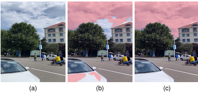
Fig. 8. A typical example showing the effectiveness of the entire refinement step. (a) An input camera frame. (b) The poor segmentation result without refinement. Note that the car below the horizon and the regions close to the building are misclassified. (c) The result with our refinement method.
