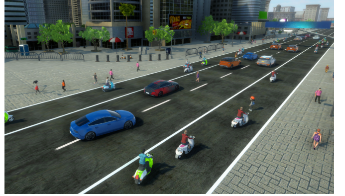
Fig. 1. Example of mixed traffic simulation result generated by our calibrated force-based approach.
