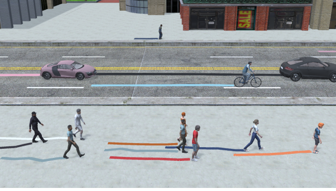
Fig. 7. Visualization of real-world traffic trajectory data which are applied to calibration of our proposed force-based model.
