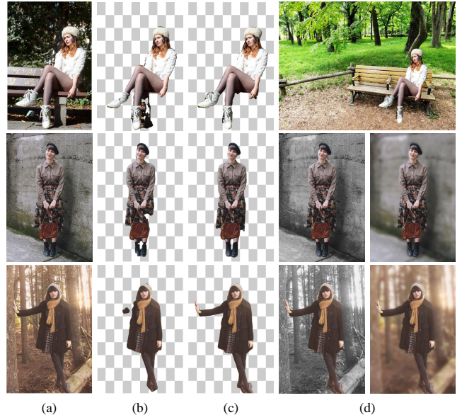
Fig. 1. Examples of the photo-editing applications benefiting from the single person segmentation. From left to right, column (a) shows input images, (b) shows segmentation results of BiSeNet [36], (c) shows the results of our approach, and (d) shows the edited images based on our segmentation results.
