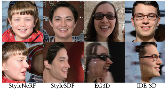
Figure 3: 3D-aware generators trained on FFHQ (StyleNeRF [12], StyleSDF [30], EG3D [5], and IDE-3D [42]) achieve excellent image synthesis performance on faces in small to medium poses (Top), but exhibit obvious artifacts at steep angles (Bottom).
