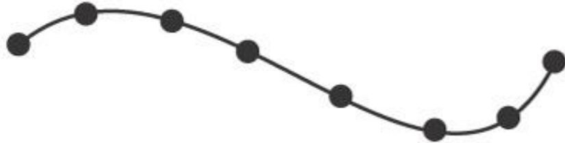
An interpolating spline in which the spline passes through the interior control points
