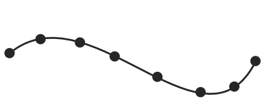
An interpolating spline in which the spline passes through the interior control points
