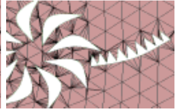
Fig.8 Interior face culling
