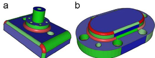
**Fig. 7.** Segmentation results of two CAD mesh models with a bit noise in the cylindrical regions. The original triangular mesh models are presented in Fig. 1, respectively.
