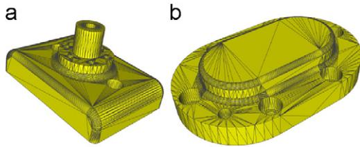
**Fig. 1.** The mesh quality of CAD mesh model is poor in the sense of mesh segmentation methods for computer graphics models, which contains sparse and dense regions. (a) and (b) are two typical CAD mesh models.
