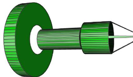
**Fig. 4.** The initial merged planar patches on the CAD mesh model after pre-processing, which are taken as the units in the Hough transformation and the followed merging operation, together with the non-merged triangular faces in the sparse region.
