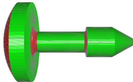
**Fig. 2.** The dense and sparse region clustering result of a CAD mesh model. The sparse region is in green, and the dense region is in red. (For interpretation of the references to color in this figure legend, the reader is referred to the web version of this article.)
