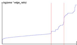
**Fig. 9.** Logarithm curve of  $\log m$  to the serials of the ordered triangles for the mesh model in Fig. 8(b). The right red vertical line is the dividing line automatically generated by the clustering algorithm, and the left red line is the dividing line selected manually. (For interpretation of the references to color in this figure legend, the reader is referred to the web version of this article.)
