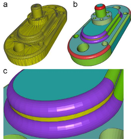
**Fig. 11.** The mean shift operation is performed on the mean curvature field to segment a dense region into sub-regions. (a) The original CAD mesh model; (b) the segmentation result; (c) zoom of the segmented dense region by the mean shift.
