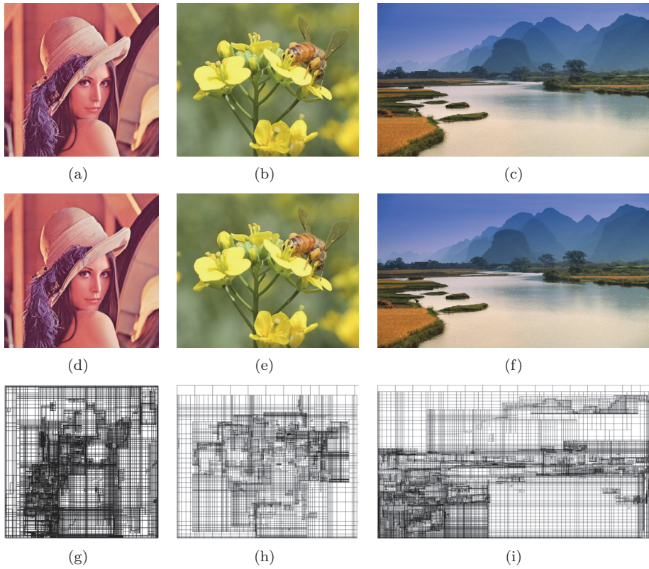
FIG. 3.5. Fitting photographic images “Lena” (left), “Bee” (middle), and “Landscape” (right) by our progressive T-spline data fitting algorithm. (a)–(c) Original images. (d)–(f) Reconstructed images from T-splines with insertion ratio 5%. (g)–(i) Preimages of T-meshes with insertion ratio 5%.
