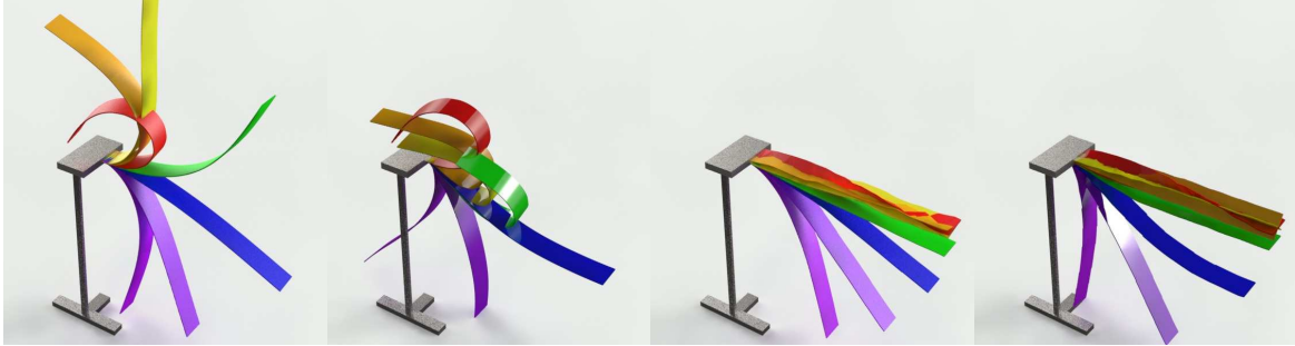
Figure 7: Results of our approach faithfully capture the dynamics of belt motion. The rainbow color denotes 7 frames sampled sequentially on a simulation sequence. Left Two: releasing a coiled belt with frames sampled on frame 1,13,25,37,49,61,73 in simulation sequence. After releasing, the left one with high stiffness swings ‘vigorously’ while the right one with low stiffness quickly collapses. Right Two: releasing a twisted belt with frames sampled on frame 1,8,16,75,125,200,250 in simulation sequence. After releasing, the left one with high stiffness dissipates twist energy quicker than the right one with low stiffness.
