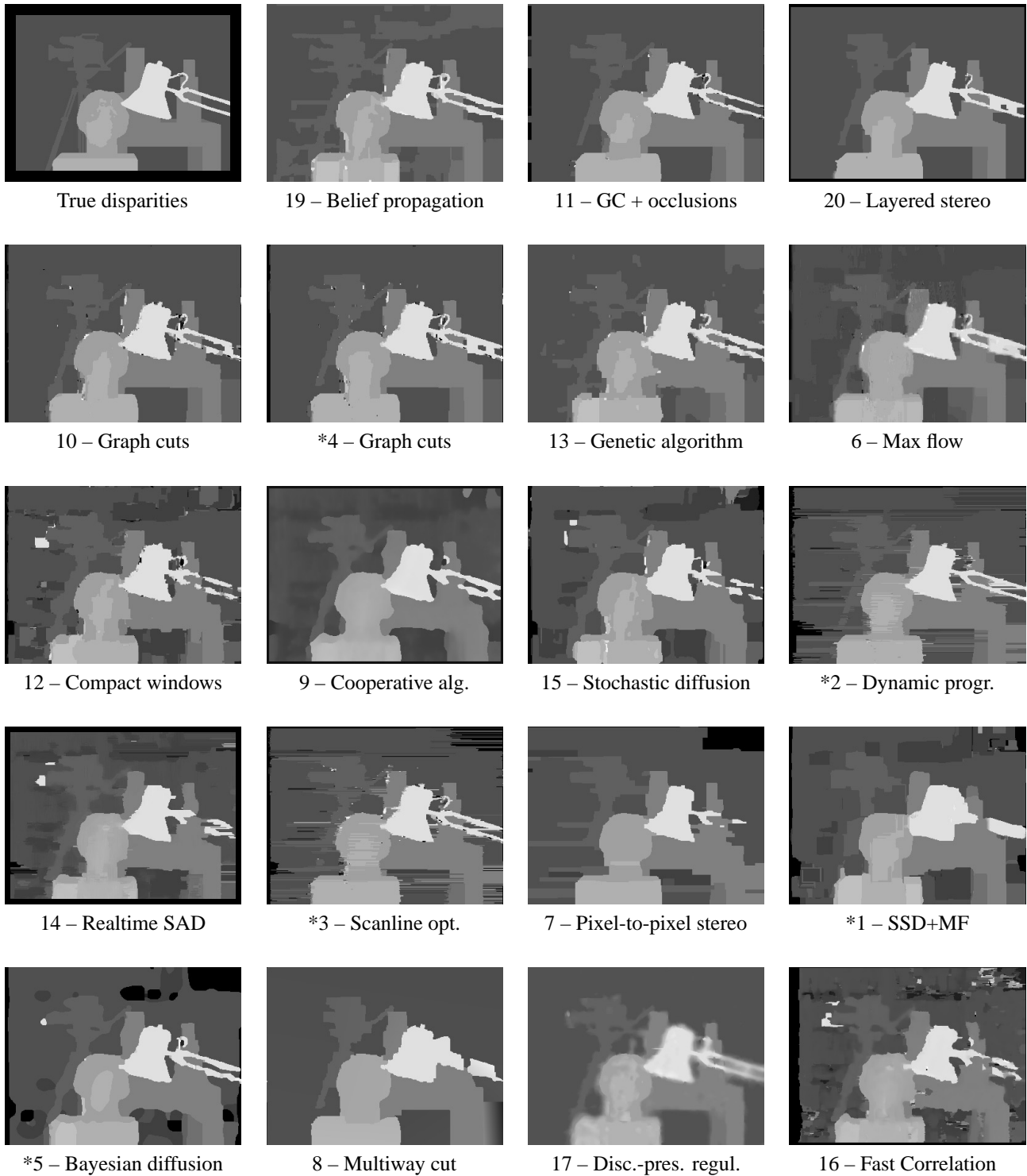
Figure 17: Comparative results on the Tsukuba images. The results are shown in decreasing order of overall performance ( B_{\overline{\sigma}} ). Algorithms implemented by us are marked with a star.
