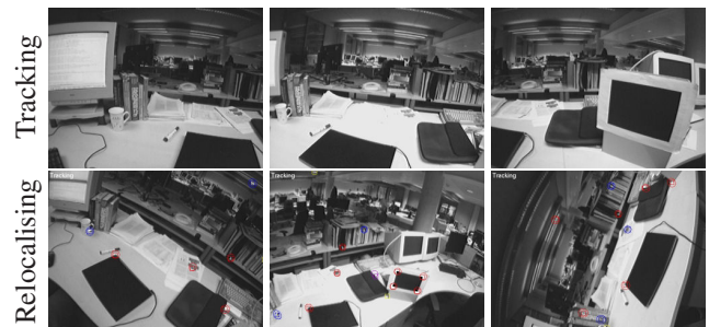
Figure 5: Relocalisation from novel views. Here tracking (and thus harvesting) was only performed along a short linear motion illustrated by the top row of images. This is sufficient to allow relocalisation from the views shown in the bottom row despite the difference in viewpoints.
