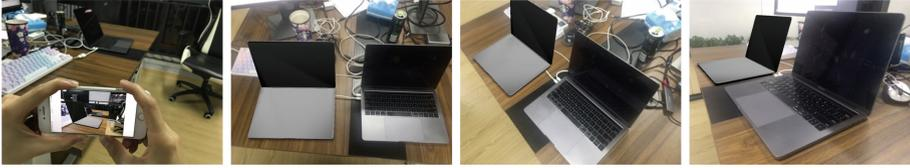
**Fig. 4.** AR effect on a mobile phone. A virtual “laptop” is placed next to the real one.
