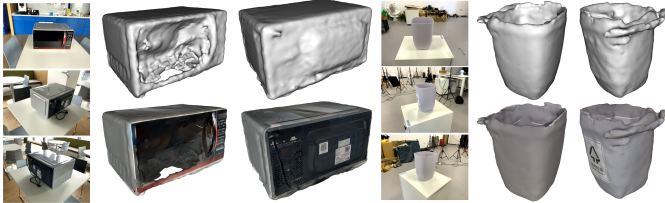
Fig. 12. Two failure cases of a microwave oven with reflecting surfaces, and a textureless trash can. Each case contains three representative keyframes, and the reconstructed 3D model with textures.
