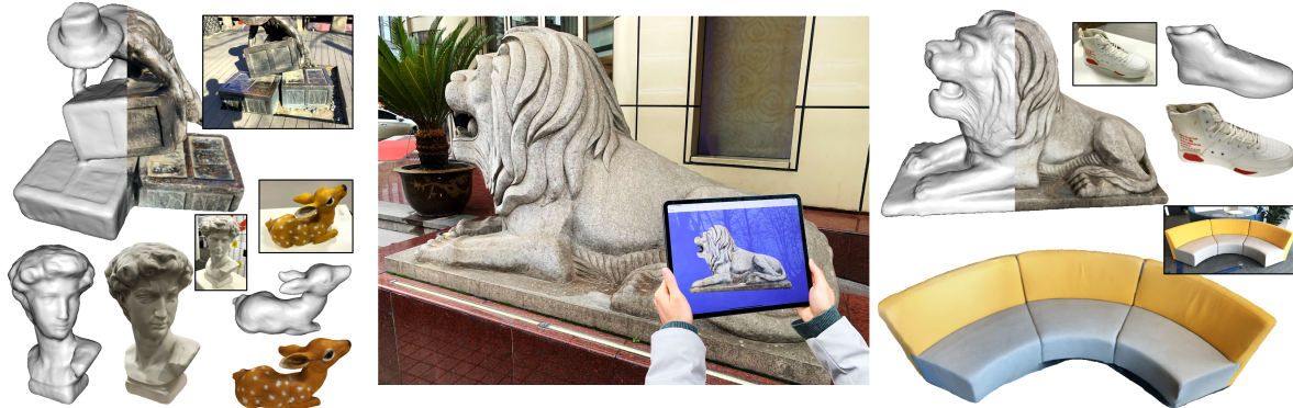
Fig. 1. Exemplar 3D models with mapped textures are shown on the left and right columns, which are scanned and reconstructed online on iPad Pro 2020 using our Mobile3DScanner system. A representative keyframe image is given for each case. As shown in the middle column, our 3D scanning pipeline is capable of scanning a large immovable object such as a “Lion” statue.
