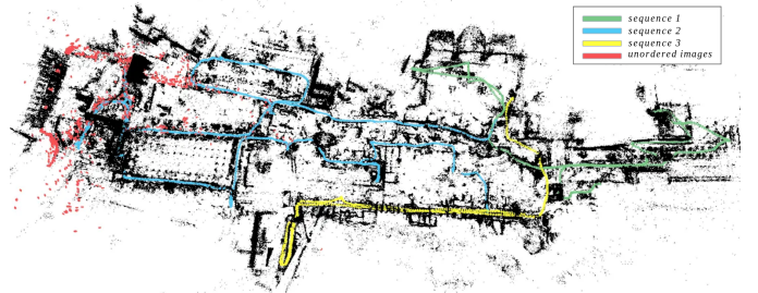
Fig. 1. The reconstruction result of Roman Forum with the proposed SfM system. Different colors distinguish different input data, including multiple image sequences and Internet images.
