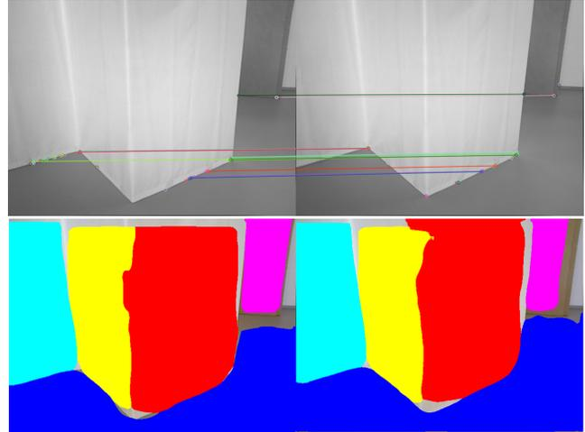
Figure 1: **Weak-texture challenge in man-made scenes.** The left shows the query image and the right shows the reference image [29]. Feature point based methods fail to extract enough matching points to group the plane (the first row) while SuperPlane (the second row) can directly detect the plane and generate the plane description. The matched planes are indicated with the same color.
