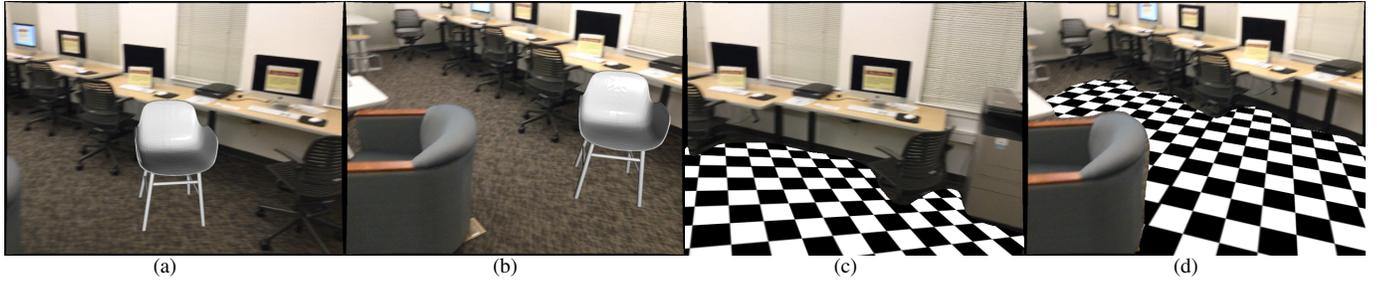
Figure 8: **Single-plane detection for AR applications.** We place the chair on the detected floor plane, as shown in (a) and (b). As the viewpoint changes, our plane can be stably detected, and the resulting plane descriptor can maintain robust tracking. We apply texture mapping to the detected floor plane, and the plane texture can be smoothly generated as the viewpoint changes, as shown in (c) and (d).
