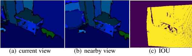
Figure 4: **Plane Description Benchmark.** We warp the current frame through a known pose to the adjacent frame, and then calculate the overlap Intersection over Union (IOU) from the current frame to the adjacent frame. The yellow part is the IOU after warping.
