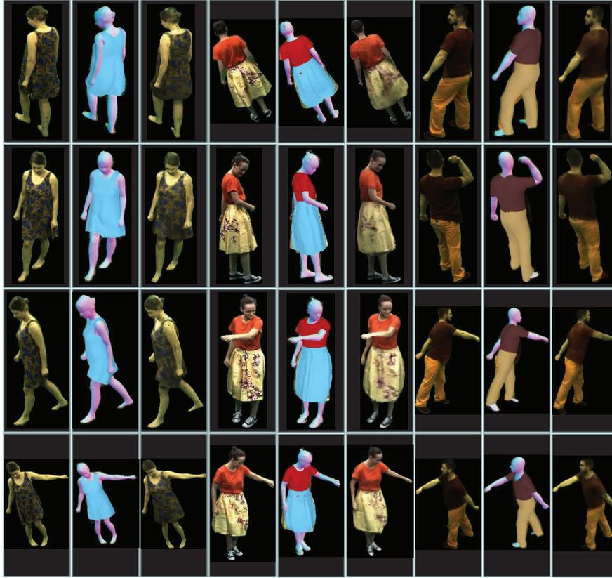
Figure 2. The results of our approach on different humans in various garments. In each example, we show the ground truth image in a novel view, the reconstructed geometry (overlaid on the image), and the novel-view synthesis image. From left to right: the S4 from DeepCap dataset [10], “FranziRed” from DynaCap dataset [8], and the S1 from DeepCap dataset [10].
