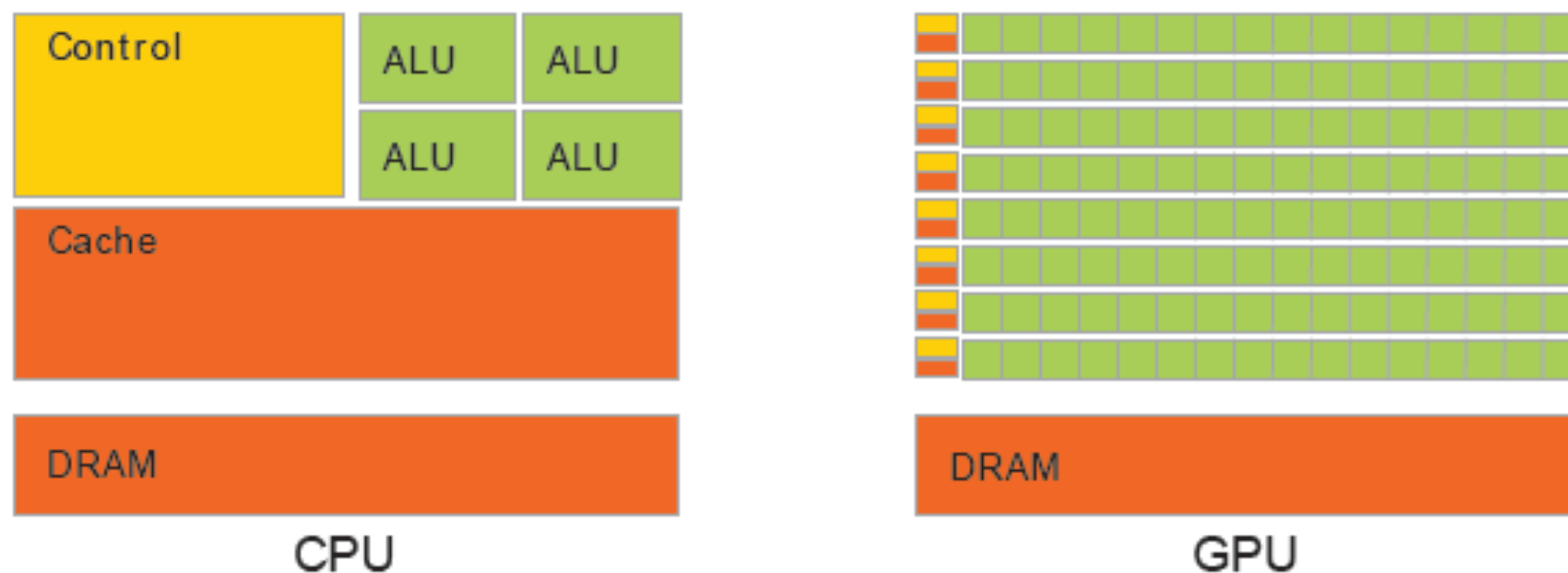
Figure 3 The GPU Devotes More Transistors to Data Processing
