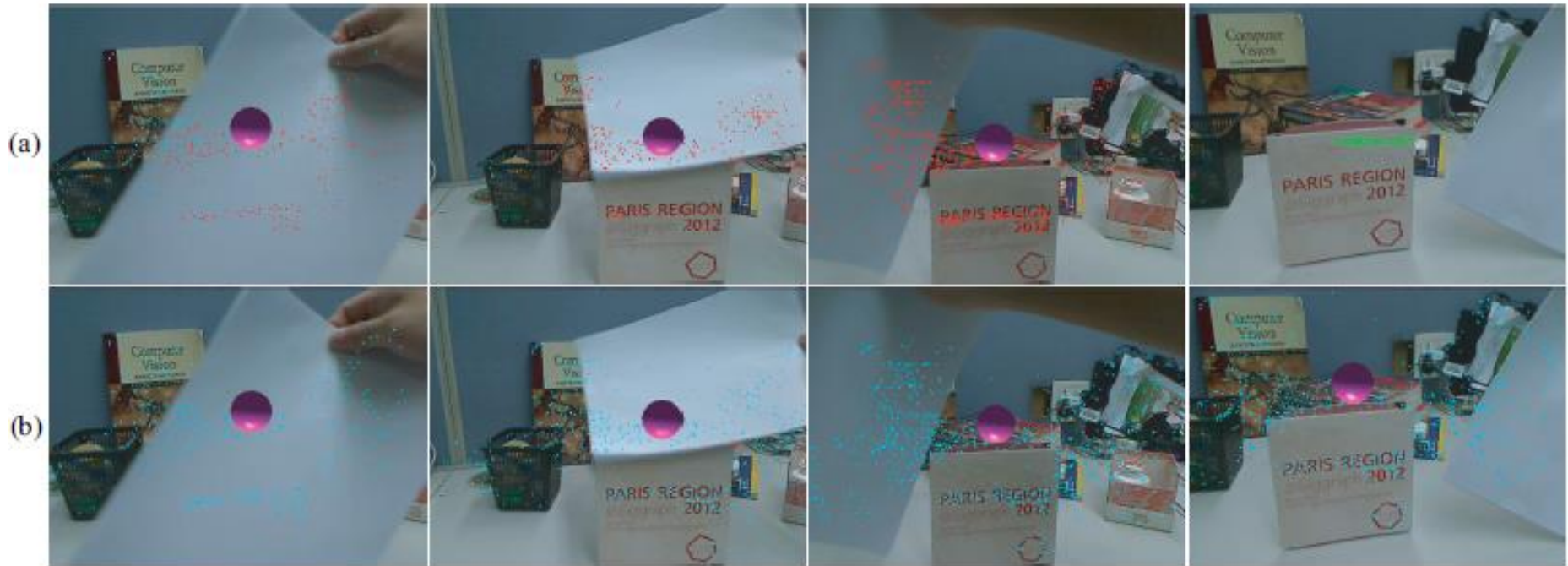
(a) The SLAM result without occlusion handling. (b) The SLAM result with occlusion handling.
